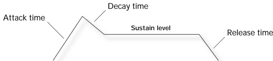
**Note:** Under its hood, FIZMO’s envelopes are actually complex 5-stage envelopes with five time and four level settings and are programmed using computer editing software. When edited from FIZMO’s front panel, envelopes are forced into an ADSR-compliant shape, and their characteristics may therefore dramatically change.
