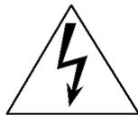
This symbol is intended to alert the user to the presence of uninsulated "dangerous voltage" within the product's enclosure that may be of sufficient magnitude to constitute a risk of electronic shock to persons.
